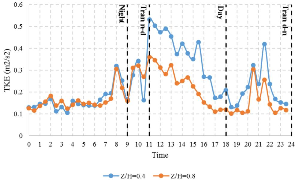
**Figure 1.** Daily TKE ( $\text{m}^2/\text{s}^2$ ) inside the canyon at  $Z/H=0.4$  and  $Z/H=0.8$ , where  $Z$  is the high of measurement level, in m, and  $H$  is the building height (20 m).
